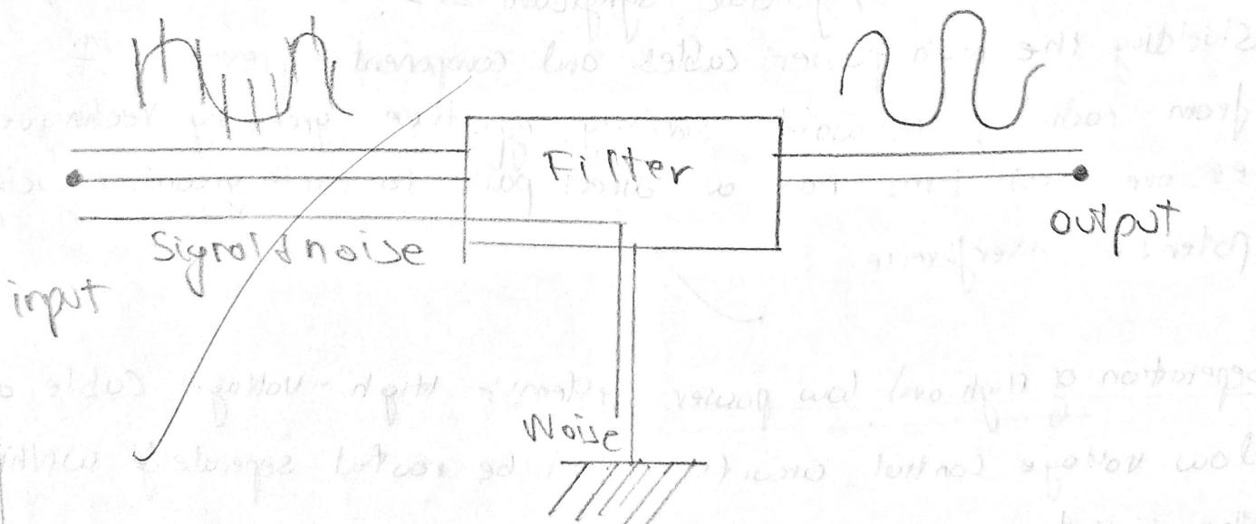
(i) a filtered power line commonly used in EV's to prevent EMI interference.
